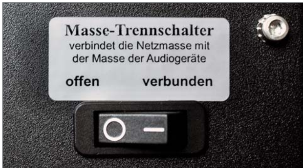
Ground lift switch
